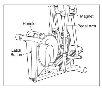
To use the elliptical exerciser, first hold the handle, press the latch button, and lower the frame.
